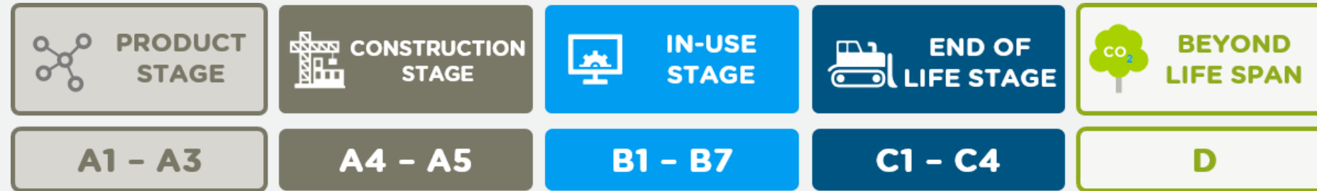
Figure 2: System Boundary: EN 15978:2011 Building Life Cycle Assessment Stages For this report, Stages A1-A4 & D (for timber) were considered
